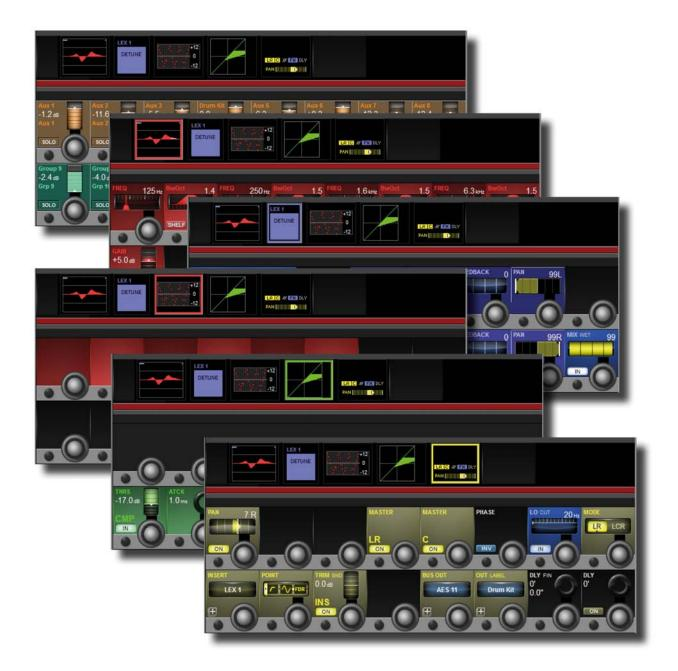
The bus output processing chain has a parametric EQ block, a BSS Graphic Equaliser block (GEQ), a dynamics block, and a Pan/Insert block. You can also label the bus, assign a physical output, and set a delay inside the Pan/Insert block.
