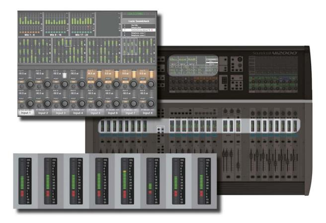
Level metering in the Vi 2000 goes from +18dB to -36 dB. It represents the actual output level in dBu from its analogue line output. Gain reduction is displayed in the Range 0 - 20dB. The Vi 2000 uses full floating-point calculations in its DSP, which means that the audio signal inside the mixer cannot be overloaded. If the signal level is too high at the master output meters, it is necessary only to pull down the master fader level until the correct level is obtained.
