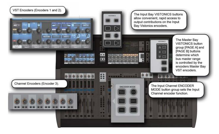
Each input channel strip contains three encoders: encoder 1 and encoder 2 are located in the VST fields in the lower screen area, while the channel encoder is located at the top of the fader area, and has an LED ring to indicate its parameter state. Each of these encoders can control different parameters, depending on the settings of other parts of the console.
