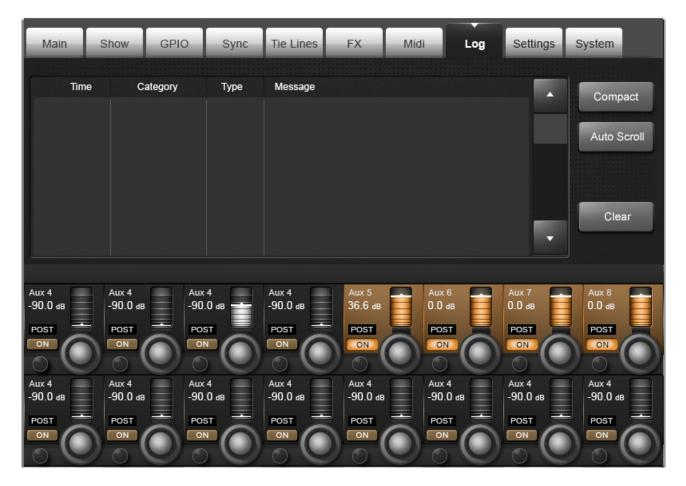
This page displays any errors that have occured since the console was last powered-up. These would usually be communications errors between the various components in the system such as control surface, local rack, and stagebox.
