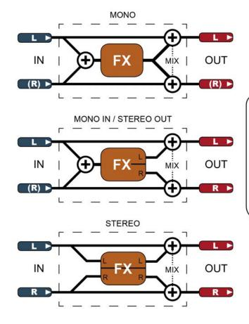
The Lexicon FX processors work in three different formats.
