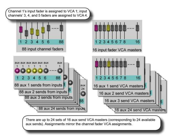
The VCA Groups on the console are normally used to control groups of the input channel faders, for use by FOH engineers. In this case they are used to group mono and/or stereo channels together under control of a single master fader, for easier control during a mix.
