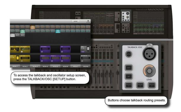
Most main oscillator and talback controls are grouped together in the master bay, though there is a Talback Assignment button [TB ASSN] in the VISTONICS button group, which allows manual assignment of the talkback group buss destinations.
