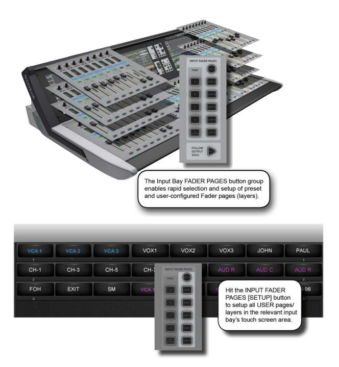
This section is used for navigating Fader Pages (or layers). There are four main layers of 24 input channel strips, and a further five user-definable layers available. The [ALL BUSSES] button maps the output busses to the input channel strips, as described further in the Outputs reference section.
