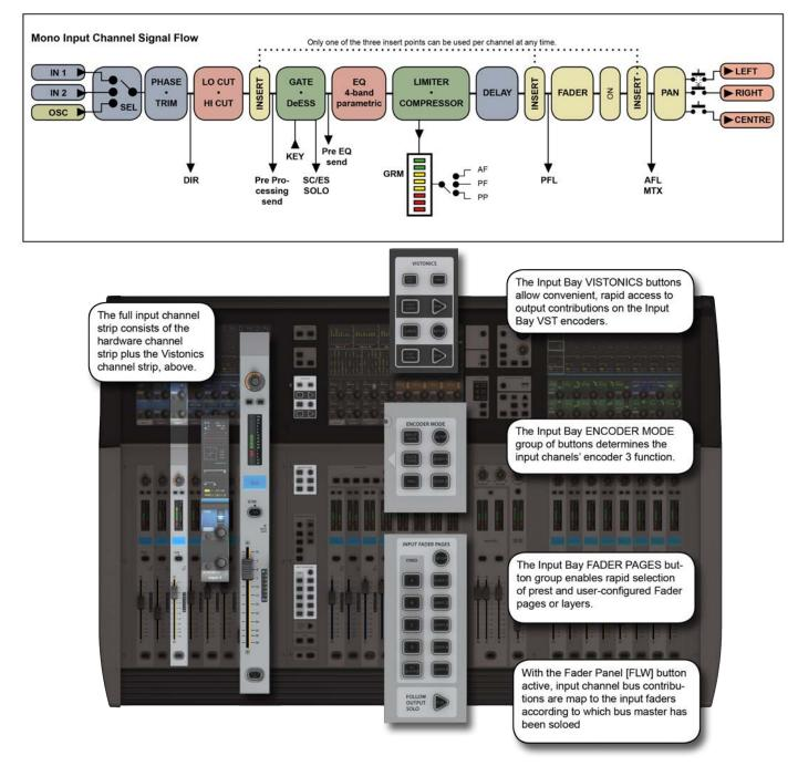
Bays 1, 2, and 4 of the console (Input Bays 1, 2, and 3) are normally dedicated to controlling input channels. However, other functions can be mapped to these channels, such as the Master Busses, Matrix feeds, Graphic EQ, and so on.
