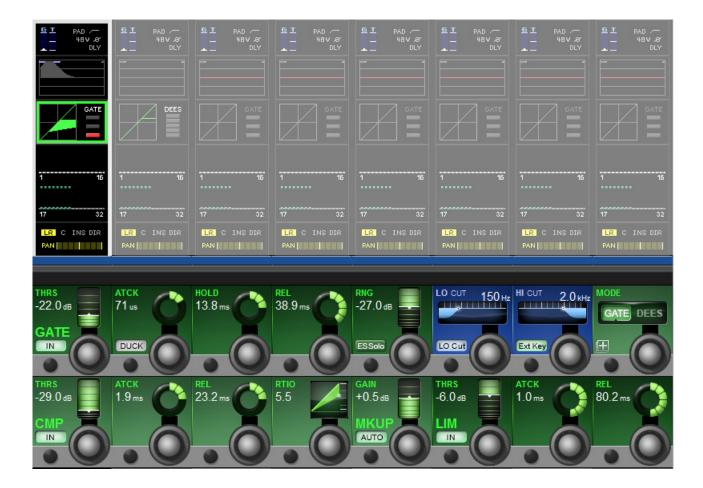
The dynamics section has three main components - The first can either be a GATE or DeEsser section; the other two are a COMPRESSOR and a LIMITER. All three sections can be turned on or off independently.
