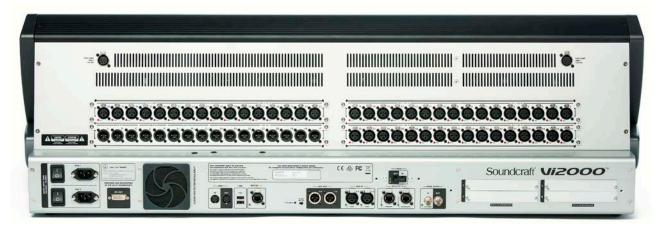
Most of the Vi2000 local I/O is located on the rear panel of the console. The main I/O slots have a variety of possible configurations, inlcuding digital (AES) and analogue input and output cards. However, the monitor / masters output section cannot be changed - this contains the fixed-routing Monitor A and Monitor B outputs, plus the master LCR analogue outputs.
