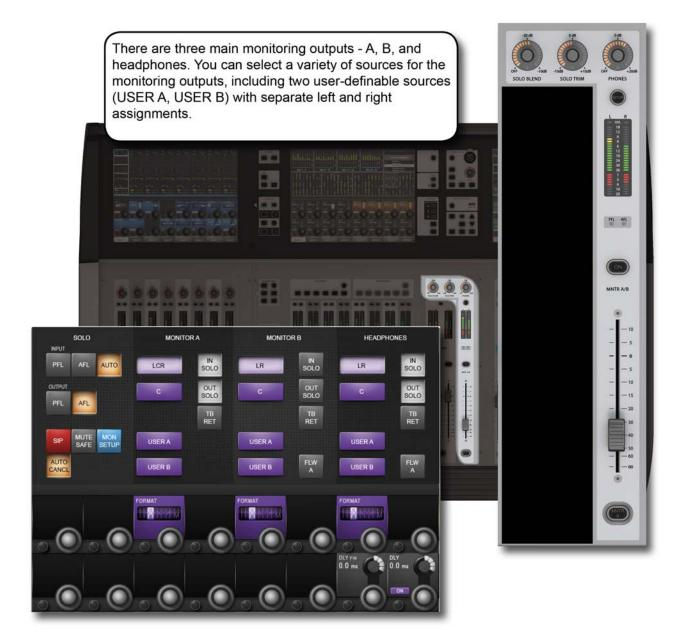
The monitoring system has three main sources - Monitor A, Monitor B, and Headphones. These are fed by a choice of sub-sources, including Solos, LCR, Talkback return, and two user-defined stereo sources where the left and right singals can be patched independently
