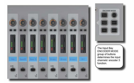
These buttons determine the function of the input channel encoder at the top of the main channel strip.
