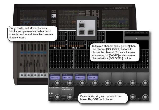
The Copy/Paste function allows the settings of any channel, bus, FX section or processing element to be copied and pasted to any number of other channels, saving set up time and helping eliminate errors.
