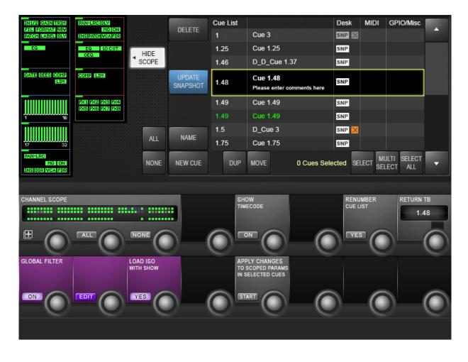
Snapshot filtering is a way of preventing certain settings on the console from changing when a Cue is recalled. There are two different reasons why this is useful, and therefore there are two different types of snapshot filtering: Global Filtering (also called Isolation), and Snapshot Scope.
