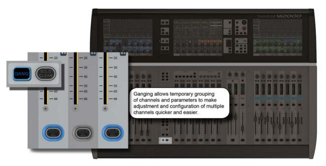
Gang is a very helpful feature to speed up operations that influence functions on multiple input channels, or on output busses, in the same way. Any parameter change on ganged channels will be applied to all other ganged channels as an offset. For example, adding 4dB of level to an aux send on one channel will add 4dB of level to the the corresponding Aux sends on all other ganged channels - it will not 'copy' the actual level to the other ganged channels.
