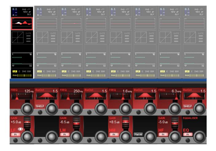
A mono input channel's parametric EQ section touch screen area is near the top of the Vistonics input channel strip area, colour-coded red. The EQ section consists of four parametric bands with shelving response available to the LF and HF bands..
