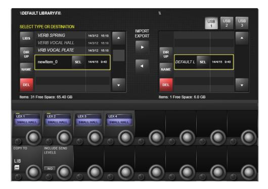
The Libraries functionality enables various elements of the console, eg EQ section, Dynamics section, or complete channels and busses, to be copied from the desk and stored in the Library system. Later these items can be retrieved and pasted from the Library to any destination channel or bus on the console. You can also export complete Libraries or individual entries to a USB stick, allowing you to move Libraries between consoles.
