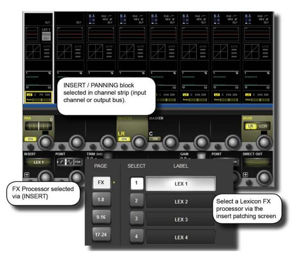
To patch an FX unit into the insert point of an input channel, select the Panning/Insert block from the bottom of the touch screen channel strip, then use the {INSERT} patch option to select an FX Unit. Touch the (FX) button on the top left of the touch screen to show the available FX selections.
