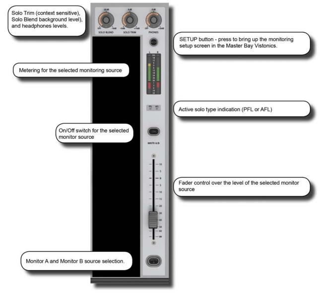
The following console monitoring controls are located to the right of the master faders in the Master Bay, except for [INPUT PRI] (Solo Input Priority), which is located with the SOLO button group on the upper section, to the right of the Master Bay.
