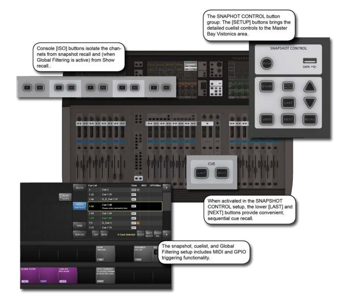
Snapshots are records of parameter settings across the console. Snapshots are stored in and recalled from cues in the cuelist. Cues can also trigger (or be triggered by) timecode, MIDI, and GPIO events. The 'scope' of a snapshot describes which parts of the console are included in the snapshot recall, and which parts are left out. Scope is set individually for every snapshot.
