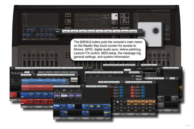
The Main Menu contains settings for general console systems and functionality, including GPIO and MIDI setup; Show loading duplicating, and export/import; Tielines (input > output patching) setup, Lexicon FX operation, and more...
