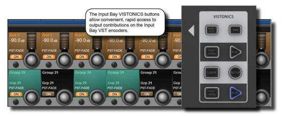
These buttons control the functionality of the input channel VST encoders.
