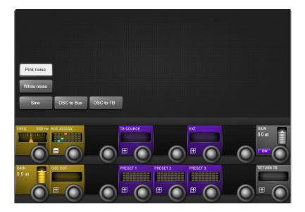
The main oscillator controls appear in the master bay touch screen area when the Oscillator / Talkback [SETUP] button is pressed. More detailed setup functions appear in the VST area, colour-coded orange.
