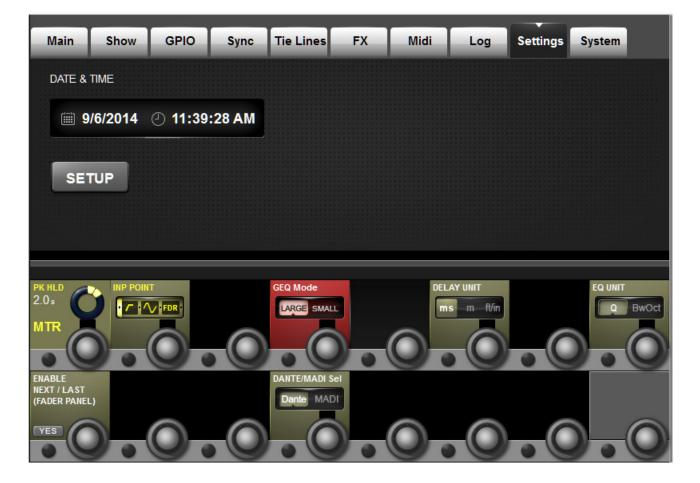
Miscellaneous settings for the console, including the date and time, plus input meter source point and general meter peak hold time, delay, EQ, graphic EQ, and Dante / MADI source selection.
