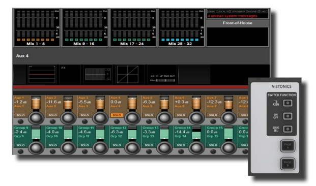
With the Bus Master Controls in the VST fields of the Master Bay, a number of primary functions are available. Use the Master Bay VISTONICS button group to control which functions and which masters are available.
