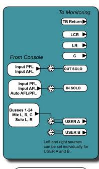
The input and output solo, and User A and User B monitor sources have their own patching options, available through the Monitoring SETUP screen.
