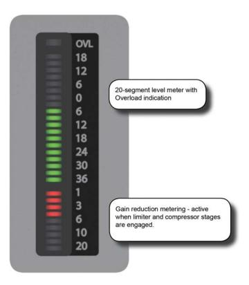
Each input channel has an input meter and every input meter has two parts: A 20--segment level meter (top), and a 9-segment Gain Reduction Meter (GRM).
