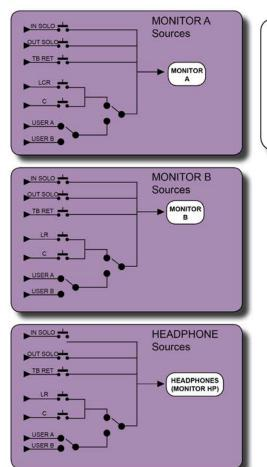
Depending on the MONITOR A, MONITOR B, and HEADPHONE (HP) source type, LCR or LR can be combined with C, though this feed and the USER A/B selection are exclusive. That is, you can choose LCR or LR and C, or USER A or USER B. Solo and Talkback return feeds can be combined with all sources.
