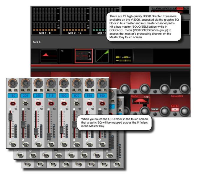
The console has a total of 27 high-quality BSS Graphic Equalisers (GEQ) - one for each of the 24 assignable Busses, and one for each of the LCR Master outputs. The GEQs are all 30-Band EQs with an adjustable bandwdith control.
