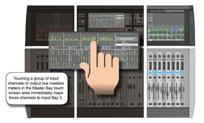
The Master Bay touch screen meters can be used as a navigation device - simply touch a block of eight meters and those channels (both inputs and outputs) are mapped to the right-hand input bay. This is excellent for fast access and for dual operator scenarios.
