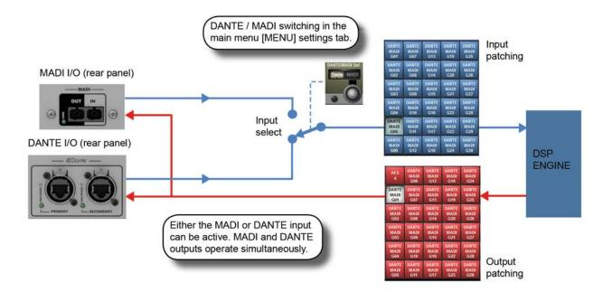
The Dante/MADI interface gives the Vi2000 a lot of flexibility for recording shows, Virtual Soundchecking or interfacing with third party MADI or Dante-enabled equipment such as signal routers or system processors.
