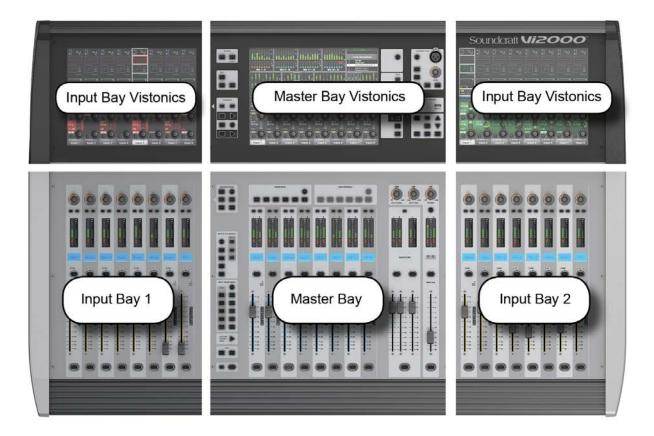
The console is divided into three main bays. Counting from the left, the first and third bays are input bays. The second bay is the Master Bay (also known as the Control Bay).
