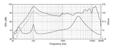
On-axis in half-space (2pi, solid line) and full-space (4pi, dotted line) at thru (8 $\Omega$ ) setting, input impedance
