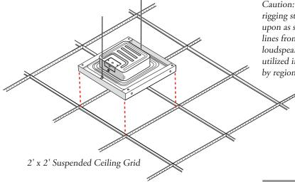
Caution: Installation must be done by qualified persons using safe rigging standards. Suspended ceiling grids can usually not be relied upon as sole support for loudspeaker. Diagram shows two support lines from suspension safety-attachment tabs on back baffle of loudspeaker. Four holes located near corners of frame can be utilized instead or in addition. Safety installation requirements vary by region. Consult a qualified installation professional.
