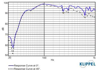
Response curves measured in anechoic chamber with the subwoofer installed in a test enclosure, 1 W / 1 m.
