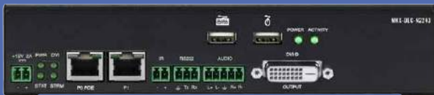
NMX-ENC-N2143 | N2143 JPEG2000 1080p60 LOW LATENCY WITH USB ENCODER NMX-DEC-N2243 | N2243 JPEG2000 1080p60 LOW LATENCY WITH USB DECODER
