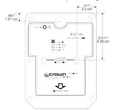
2. Using the supplied small screwdriver, turn the pot clockwise for high-frequency boost (a brighter sound); turn the pot counter-clockwise for high-frequency rolloff (a duller sound).
