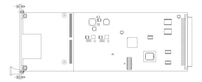
DIP Switch: S1 DIP switch for D21m channel count setting:
