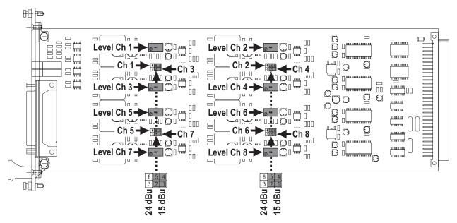
Jumpers: Level (Ch1...8) Two positions each: 15 dBu (factory default) or 24 dBu.
