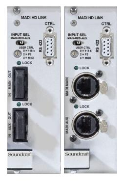
The MADI HD card is plugged into the HD card slot in the Stagebox and provides the link to the Local Rack frame. The two interfaces offer up to 64 audio channels with 48kHz operation, together with embedded control and user-accessible serial connection in each direction.
