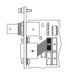
If the meta data of both decoder modules is required, plug the short flat cable (W1) coming from the METADATA OUT front-panel socket to the PCB socket P4 (labeled META1+2).
