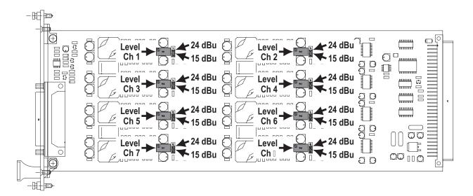
Jumpers: Level (Ch1...8) Two positions each: 15 dBu (factory default) or 24 dBu.
