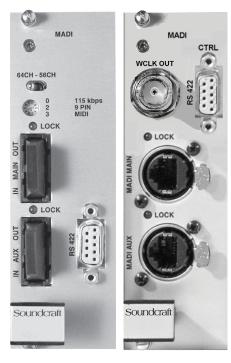
The MADI I/O card can establish a 64-channel MADI input and output to the stagebox or other equipped device. Optical inputs and outputs are provided on SC connectors available in multi-mode and single-mode versions, as well as a version with RJ45 connectors for twisted-pair cable and an additional word clock output on a BNC socket.
