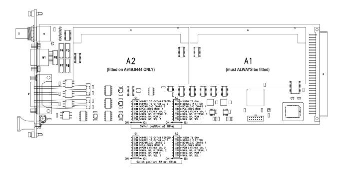
LEDs: M1 / M2 Indicates that a valid AES/EBU signal is detected on main input 1/2.
