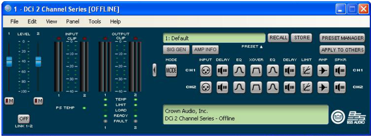
Figure 14 (above) shows the DriveCore Install 2 channel configuration page. The 4 and 8 channel amplifier configuration pages have the same feature set. The DriveCore Install Network amplifier includes Digital Signal Processing (DSP), multiple input/output routing options and a comprehensive diagnostics feature set. All of these features can be adjusted in from the configuration page.
