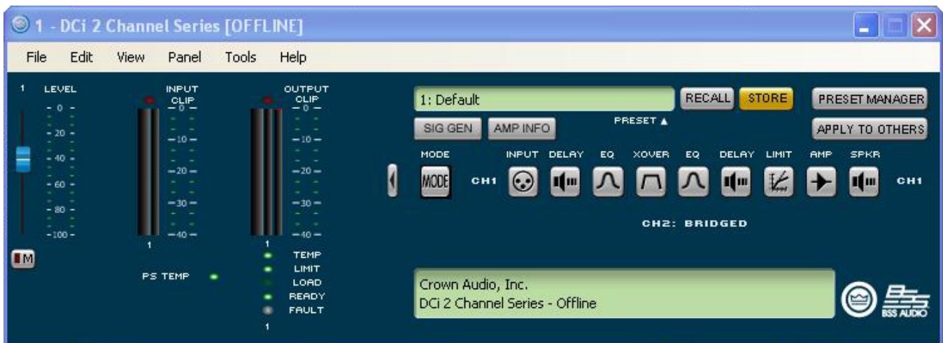
Figure 19 By selecting Mono Bridge output, only one channel in the channel pair DSP will be available.
