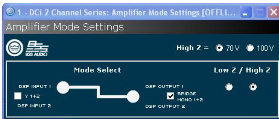
Figure 27 Operation mode for 140Vrms or 200Vrms.
