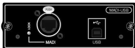
MADI-USB (32 in/ 64 out MADI + 32 in/out USB, OR 64 in/out MADI + 32 USB out only. Connect Soundcraft Stagebox plus a PC or Mac. See section 5.4 for more detail.
