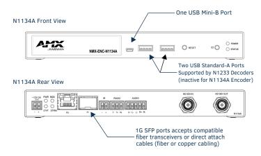
FIG. 1 N1134A USB AND SFP PORTS
