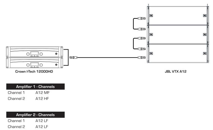
**TIP:** Other channel assignments can be implemented when using the 2-channel Crown Audio I-Tech HD amplifiers. Use JBL's HiQNet <sup>®</sup> Performance Manager<sup>™</sup> control software to assign speaker presets.
