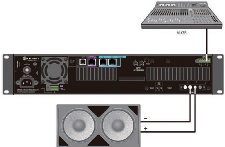
Figure 13 System Wiring Bridge Mode
