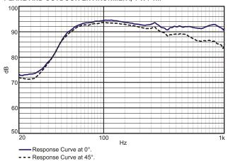
Response curves measured on ground plane and outdoor environment with the subwoofer installed in a test enclosure, 1 W / 1 m. This curves was decreased 6 dB to compensate the ground plane gain.
