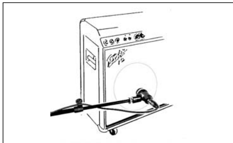
Fig. 3: Microphone placement for a guitar amp.
