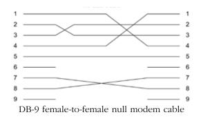
Important Note! A straight through RS-232 cable will not work with the DriveRack.
