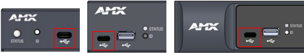
FIG. 9 USB-C Program port On MU-1000 (Left), MU-1300 (Center), and MU-2300/3300 (Right)
