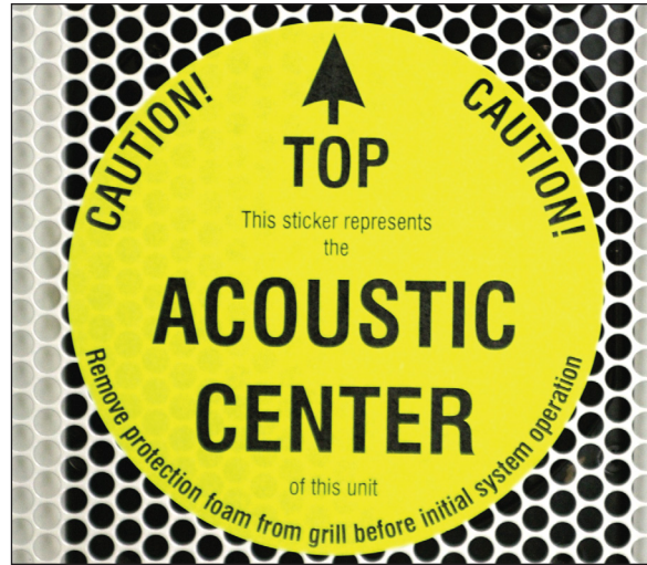
fig.12 Sticker showing acoustic centre and unit orientation
